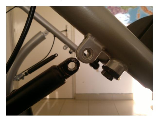
12. Insert screw M8x30 with the head from the inner side.
