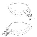
Disassemble and change the seat support by unlocking the two screws according to picture. Use the attached screws to assemble the new seat support and please note that there is a left and right seat support.
