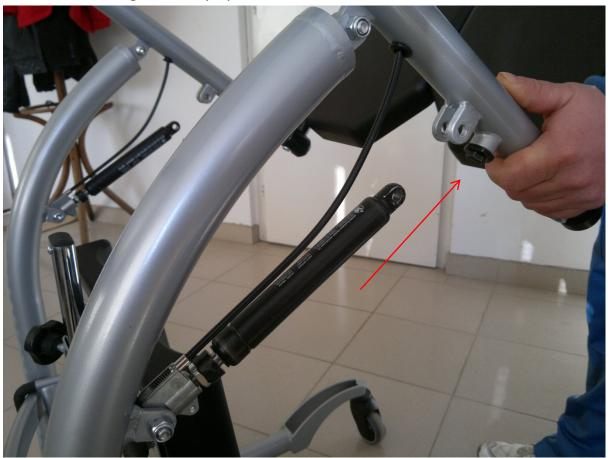
6. Unscrew the gas pistons if they are in the outermost position.
