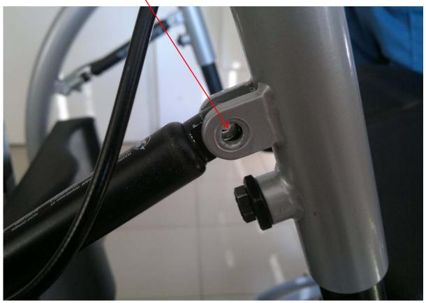
4. Loosen two securing nuts on each piston.
