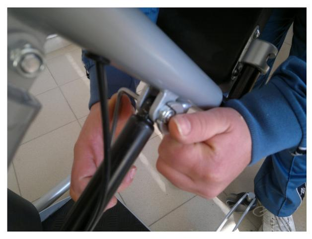
That was the last step towards this standard adjusting procedure. Now the VanMove should function properly. If one of the gas pistons start to extract sooner, it could be fine tuned by turning the aluminum adjusting barrels.
